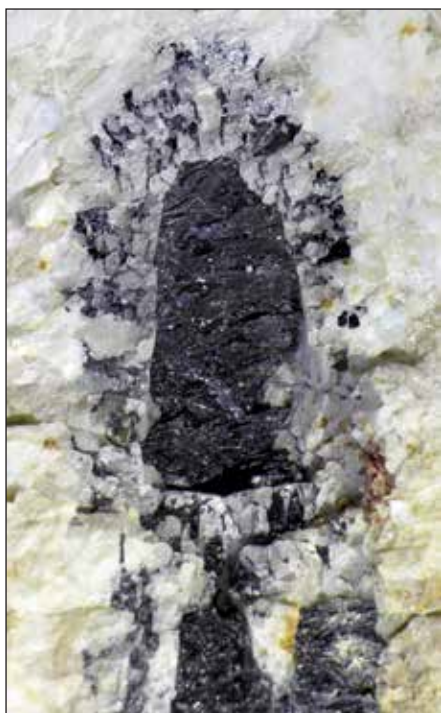
Figure 112. Black tourmaline aggregate (schorl) similar to the ones illustrated in Figures 110 and 111. This picture better illustrates the rim of the aggregate, composed of a relatively fine-grained texture of tourmaline and quartz.
