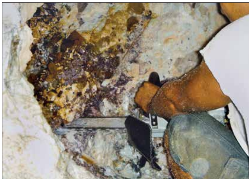
Figure 242. Cutting specimens out of Burkhard's Pocket with the diamond chain saw. José Menezes photo.
