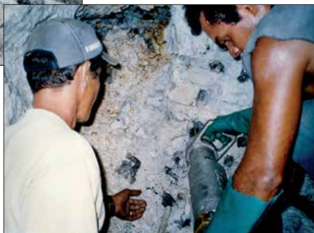
Figure 30. Miners using the pneumatic rock splitter to carefully break apart the pegmatite without causing shock waves that could damage crystals inside.
