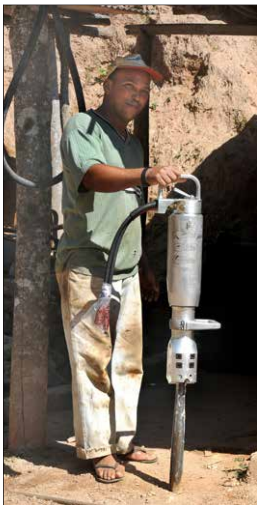
Figure 81. Elci with the pneumatic rock splitter used for gently opening pockets. Andrea Dini photo.
