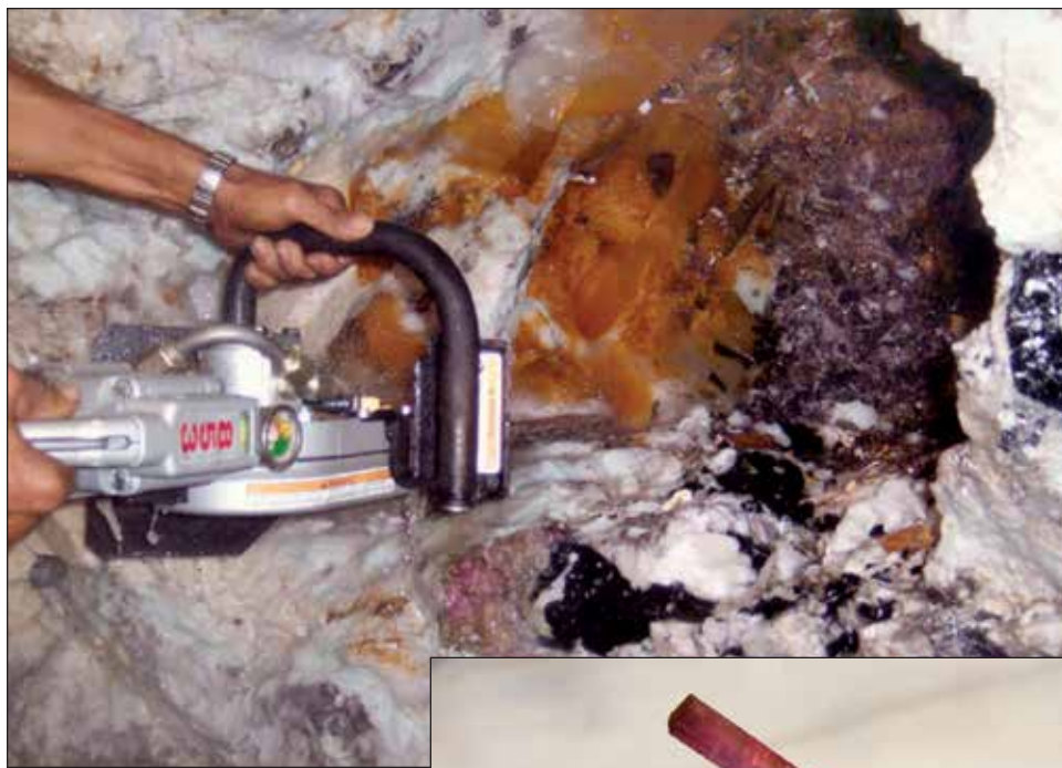
Figure 38. Removing matrix pieces from the Grandon Pocket using the diamond chain saw.
