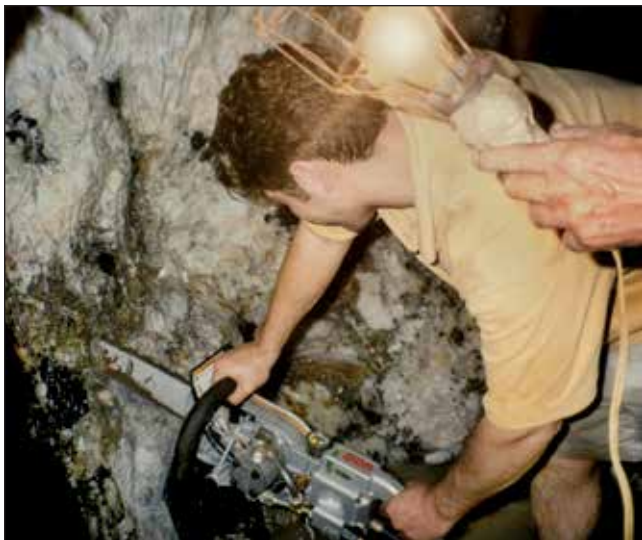
Figure 34. Demonstrating the use of the diamond chain saw for removing crystal pockets (2001).
